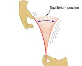
Figure 16.2 When displaced from its vertical equilibrium position, this plastic ruler oscillates back and forth because of the restoring force opposing displacement. When the ruler is on the left, there is a force to the right, and vice versa.
