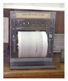
Figure 16.48 A seismograph as described in above problem.(credit: Oleg Alexandrov)
