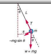
**Figure 16.14** A simple pendulum has a small-diameter bob and a string that has a very small mass but is strong enough not to stretch appreciably. The linear displacement from equilibrium is *s*, the length of the arc. Also shown are the forces on the bob, which result in a net force of  $-mg \sin\theta$  toward the equilibrium position—that is, a restoring force.
