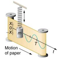
Figure 16.11 The vertical position of an object bouncing on a spring is recorded on a strip of moving paper, leaving a sine wave.
