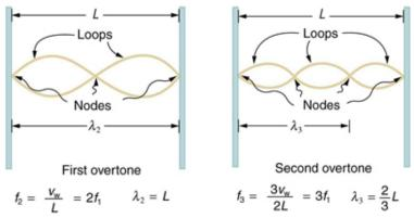
Figure 16.41 First and second harmonic frequencies are shown.
