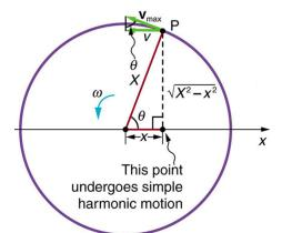
Figure 16.19 A point P moving on a circular path with a constant angular velocity  $\omega$  is undergoing uniform circular motion. Its projection on the x-axis undergoes simple harmonic motion. Also shown is the velocity of this point around the circle,  $v_{max}$ , and its projection, which is v. Note that these velocities form a similar triangle to the displacement triangle.
