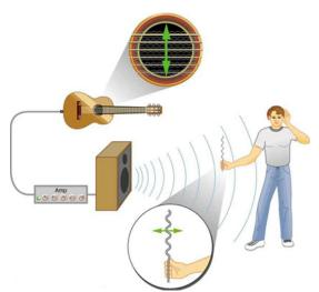
Figure 16.33 The wave on a guitar string is transverse. The sound wave rattles a sheet of paper in a direction that shows the sound wave is longitudinal.
