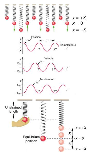
Figure 16.12 Graphs of x(t), v(t), and a(t) versus t for the motion of an object on a spring. The net force on the object can be described by Hooke's law, and so the
