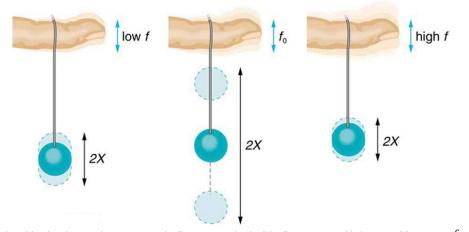
Figure 16.26 The paddle ball on its rubber band moves in response to the finger supporting it. If the finger moves with the natural frequency  $f_0$  of the ball on the rubber band, then a resonance is achieved, and the amplitude of the ball's oscillations increases dramatically. At higher and lower driving frequencies, energy is transferred to the ball less efficiently, and it responds with lower-amplitude oscillations.
